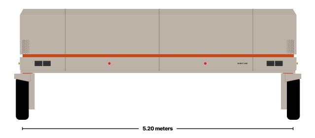
40 high-power lasers Can mount up to 4 laser units, 10 lasers per row
